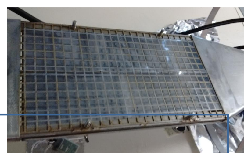
SR strips exposed to the seawater within a drum constantly flushed by seawater (Atlantic)
