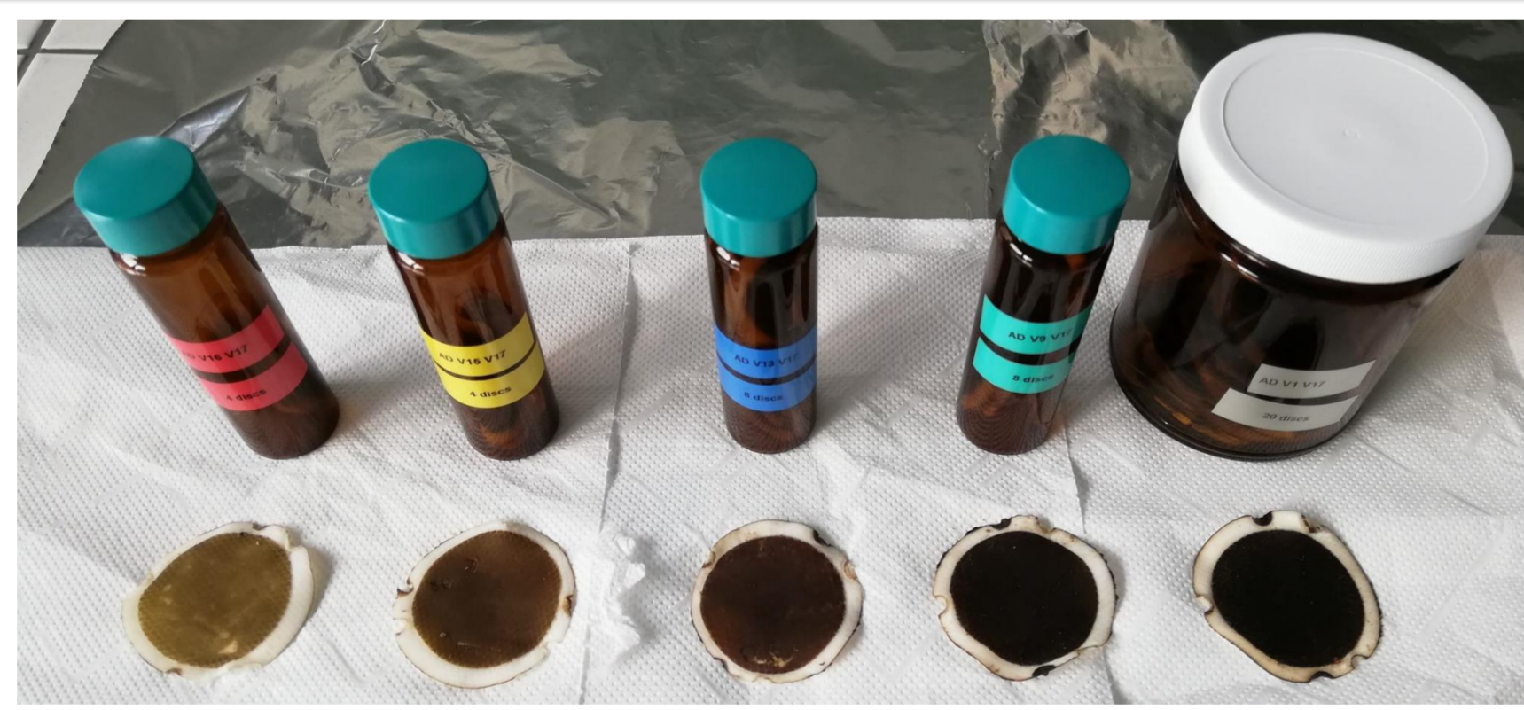
HLB disks after 1, 2, 4, 8 and 16 weeks exposure in effluent of WWTP Modřice
