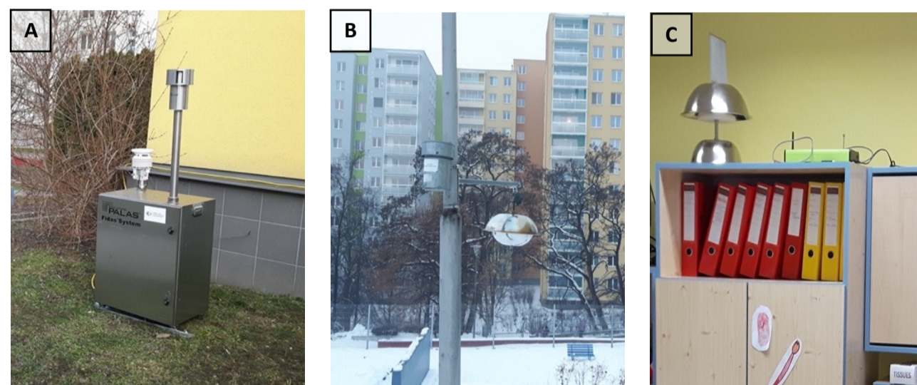
Figure 2: A) active air sampler Palas Fidas 210S, B) passive air sampler with PUF disks, disks are closed for outdoors use, C) passive air sampler with PUF disk, disks are opened for indoors use and GRIMM Mini Laser Aerosol Spectrometer, model 11E
